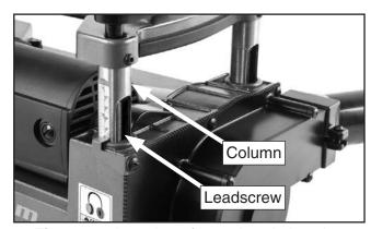
**Figure 24.** Location of cutterhead elevation leadscrews.
